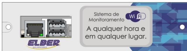
The Wi-Fi module allows the monitoring of the system via the Internet. Allows you to obtain reports, system information and register mobile numbers and emails to be notified in case of problems, all through a computer with internet access.
