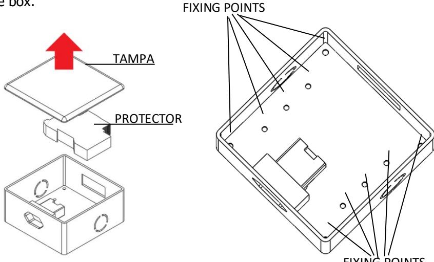
To secure the DPS Kit housing, simply position it to the desired location and insert the screws through the attachment points.
