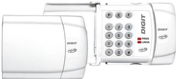
The tele alarm works through a telephone line. Makes calls to the numbers recorded when the temperature drops out, or if the battery voltage is low. For the dialer to work, you need to connect a telephone cable.
