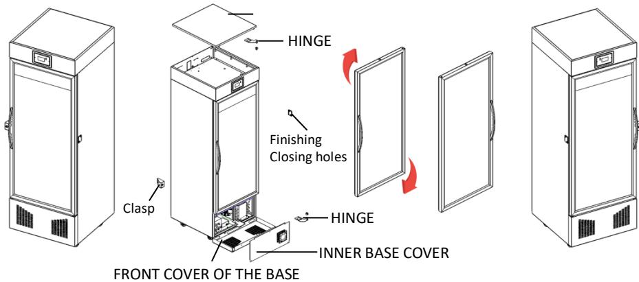
(\*) For conservatives who have a lock on the door, they will be prepared to meet the inversion of the door opening as well, just remove and install the clasp and finish the holes on the other side of the conservative.
