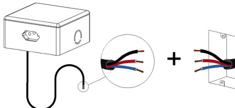
**WARNING:** The correct insulation of the wires is indispensable, either by an insulating tape or retractable thermo spaghetti.
