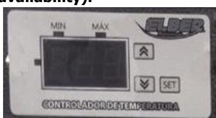
The V2.7 controller continuously records the lowest and highest temperature reached by the sensor. To check the recorded temperatures, press the key for the maximum temperature,
