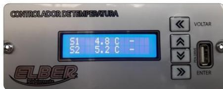
The first sensor will represent the temperature inside the conservator. When it has two sensors, the second sensor will represent the temperature inside the glycerol tube, which simulates the temperature of the stored material.
