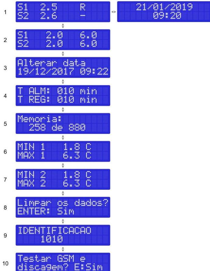
Menu 1 toggles between sensor temperatures and the date / time every 2 or 3 seconds. The letter "R" indicates that the compressor is on.
